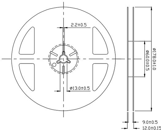
**Carrier Tape Dimensions: Loaded Quantity 2000 pcs Per Reel**
